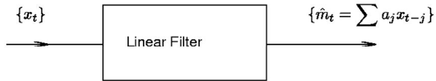
Figure 1-20 Smoothing with a low-pass linear filter.
